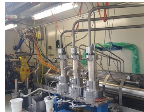
Fig. 1 – Ethanol tests at ERIC (Switzerland): RTX-6 engine, Test rig, and Spray Combustion Chamber with lab scale prototypes
