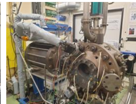
Fig. 1 – Ethanol tests at ERIC (Switzerland): RTX-6 engine, Test rig, and Spray Combustion Chamber with lab scale prototypes
